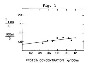
The line, fitted by the method of least squares, gives an intrinsic viscosity of about 0.036 dl/g. This value is in the same range as that reported for bovine serum albumin, a globular protein, and indicates that the G-ADP actin is 1 mg/ml this actin preparation polymerized at 30°C to give a reduced viscosity of about 5 dl/g at a rate of shear of approximately 1900 sec-1.
